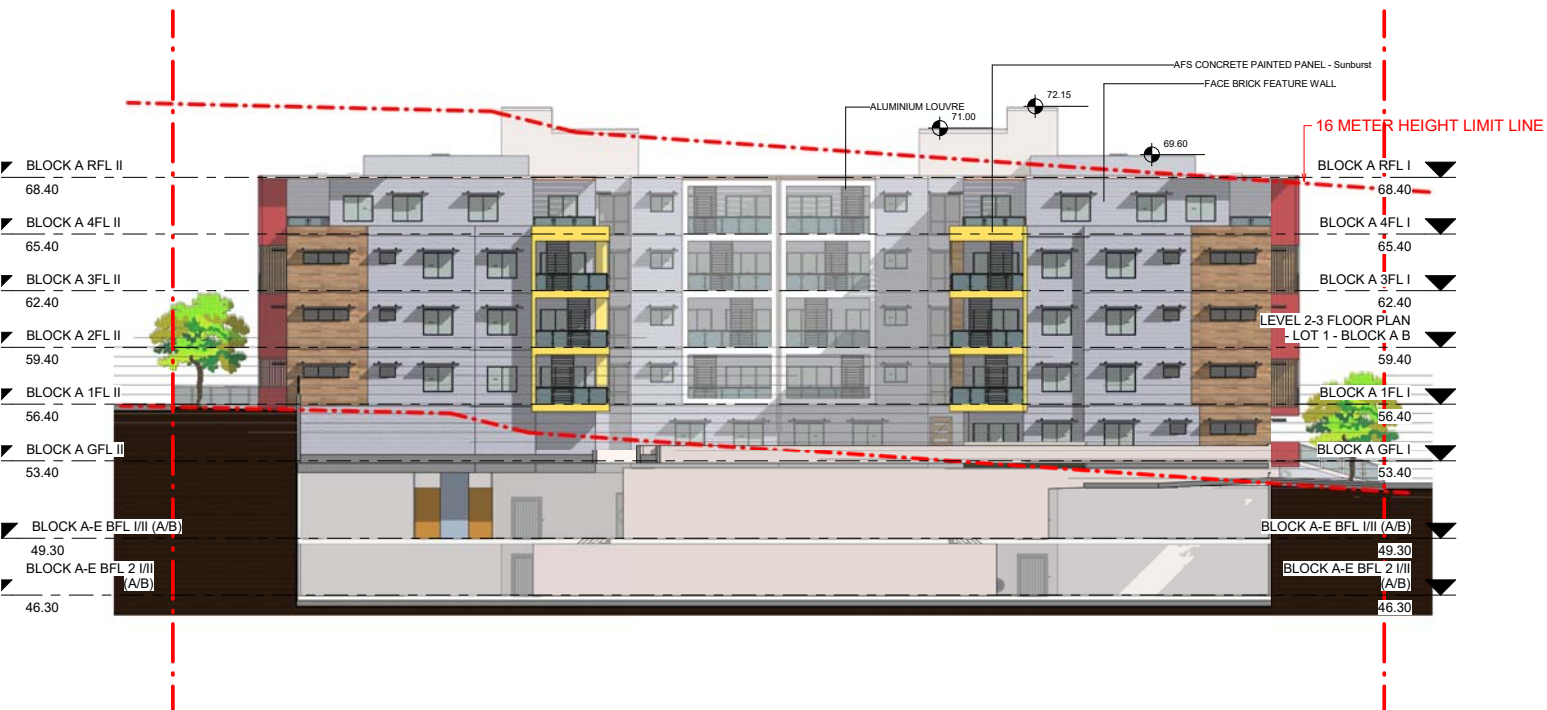
1 EAST ELEVATION BUILDING A 1 : 200 @ A1
